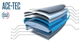
1- Deck Pad. / 2&10- Thermoformed plastic skin (ASA). / 3- 50g/m² Fiberglass wrap. 4&8- 200g/m² Woven Fiberglass. / 5- 200g/m² Woven Fiberglass Reinforcement Patch in standing area. / 6-200g/m² Woven Fiberglass Rail Reinforcement. 7- Molded, Watertight EPS Foam Core. / 9- 50g/m² Fiberglass wrap.
